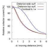
Fig. 2. Characteristics of the Everlight ITR8307 proximity sensor measured against printed plastic surfaces. The distance measurements were taken against the side (black) and top (red) of a white 3D-printed object to evaluate the effect of differently textured surfaces.
