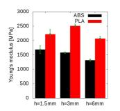
Fig. 4. Young's modulus measured from the 1.5, 3.0 and 6.0m m high beams of ABS and PLA.
