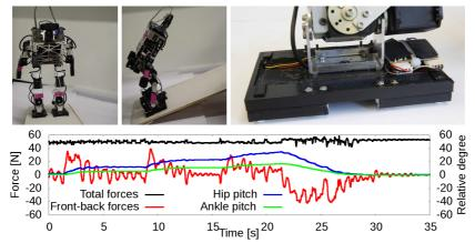
Fig. 6. The Hambot robot while adapting to a tilted ground (left and center), 3Dprinted foot of the robot with four force sensors enclosed by light shielding hulls at each corner (right). Force sensor data and the rotation of the pitch motors while the robot is balancing and adapting to the tilted ground (bottom).
