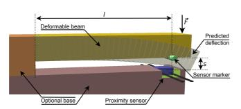
Fig. 3. OpenSCAD rendering of the basic one dimensional push-force sensor, with the deformable beam on top and above the optical proximity sensor. To help the designer to dimension and align the sensor, the rendering optionally also includes the sensor marker (green), the fully deflected beam (gray), and a model of the proximity sensor (blue).
